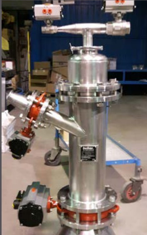
-BTS- Bulk transfer system
